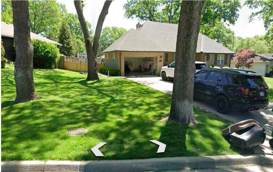
5203: JCW MH , 3 feet from the back of curb Healthy Ash Tree with exposed roots 4 LF from B/C, diameter 25" Would not be able to continue along BOC
