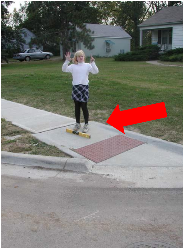
Figure 10b – Measuring Longitudinal Slope
