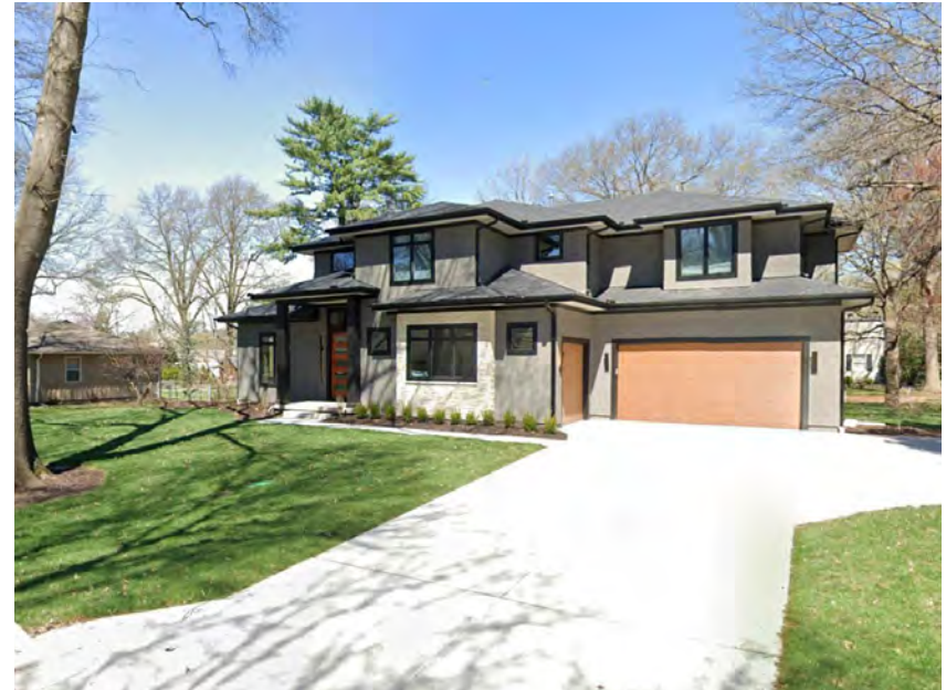
Figure 5.1 - Example of appropriately scaled and setback garage
