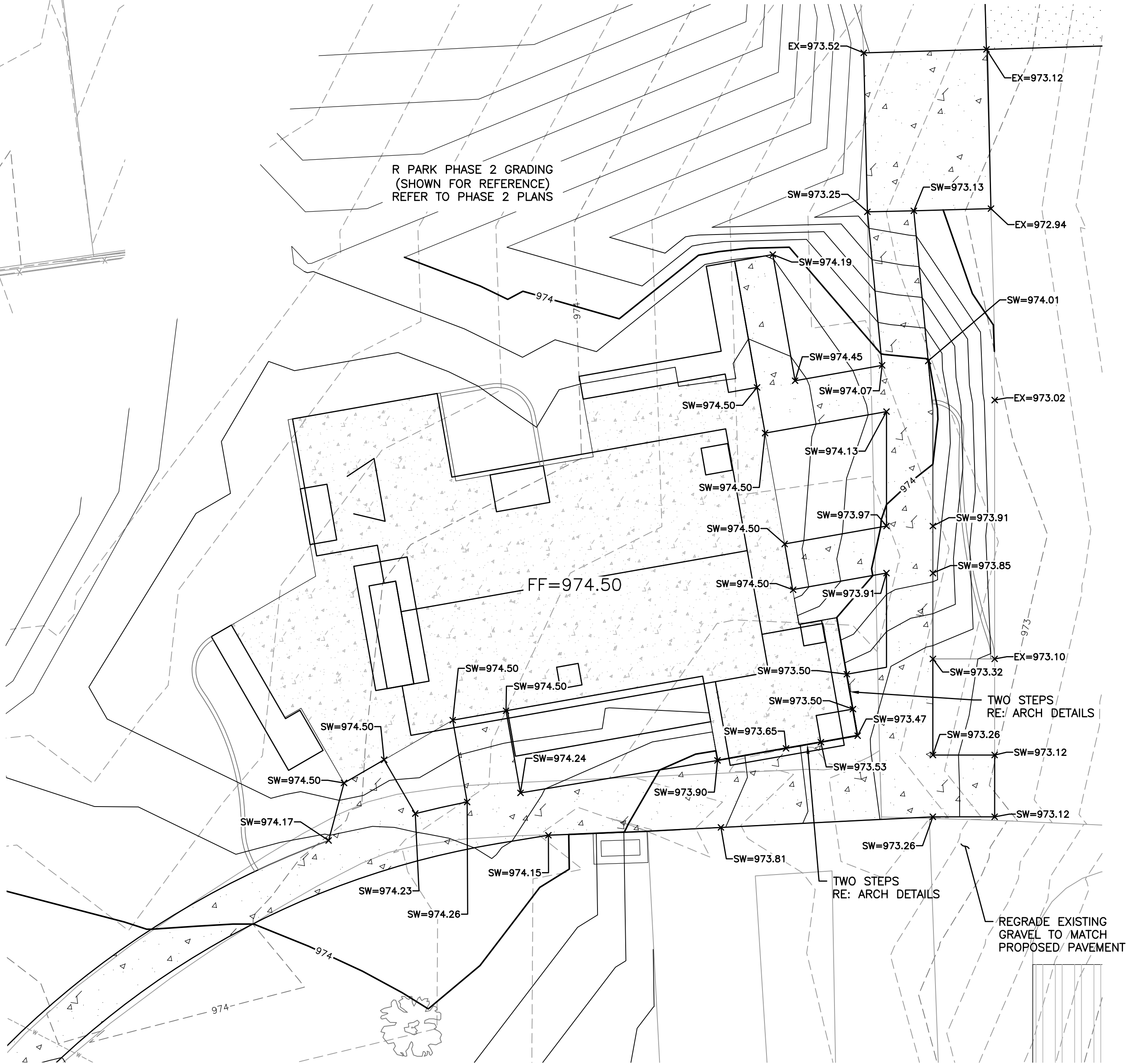
PAVILLION GRADING PLAN
